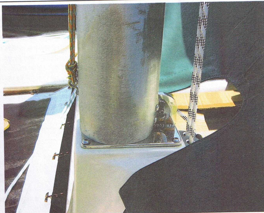
Mast step integrated into the mast beam is a new feature on the 8 metre, as are deeper section crossbeams.
